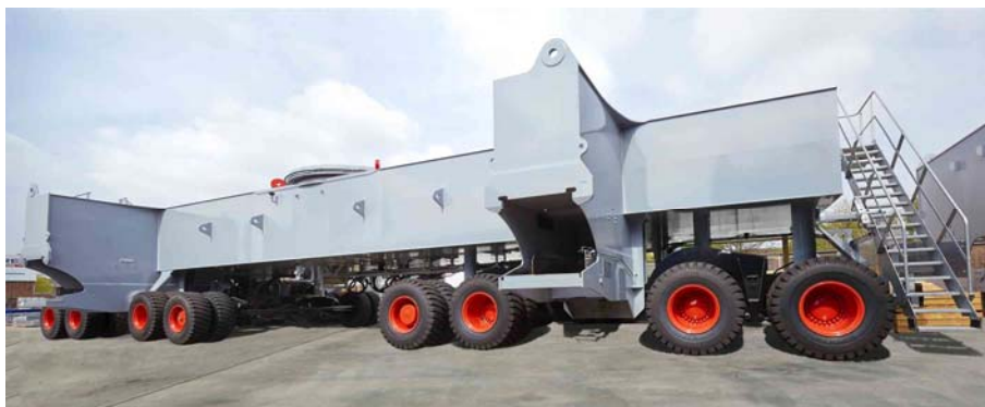
In order to meet the specific conditions of the quays, the two G HMK 6408 cranes for Napier Port will be equipped with 8-axle chassis – seen here during assembly at the Terex Port Solutions plant in Düsseldorf
