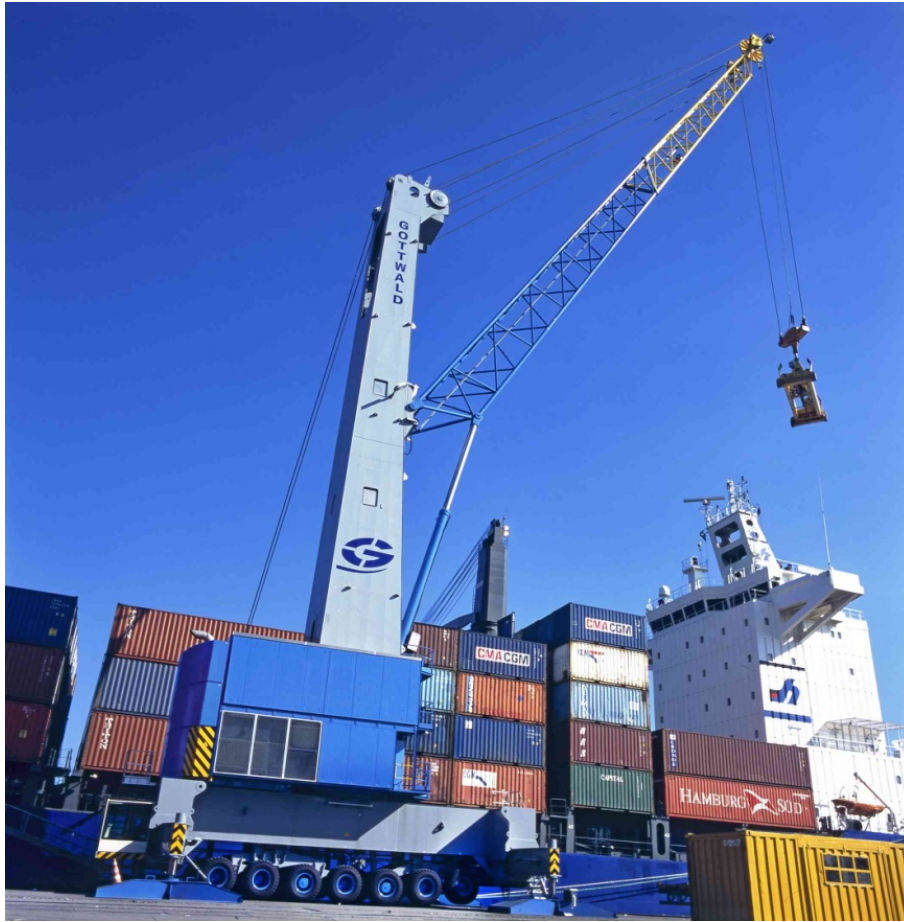
Terex Gottwald G HMK 6407 mobile harbour crane with standard 7-axle chassis handling containers
