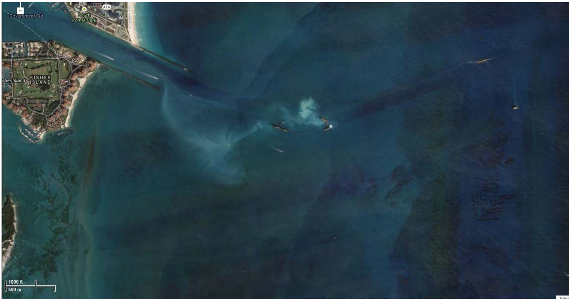
Figure 7. Aerial photo of current dredging (adopted from Google Maps in July of 2014). The length of turbidity plume is over 1500 m westward and 1000 m southwestward. There were no documented turbidity violations at this time according to project data.
